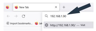
The Web UI is available on HTTP port 80, if you know the IP address of the gateway, simply enter "http://<IP Address>" into the address bar of your web browser (e.g. http://192.168.1.90).
