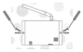
The gateway is fixed by using plastic anchors and Phillips screws to the wall or solid surfaces of suspended ceilings making sure that it is in a good radio position for receiving and transmitting signals. When located in shielded surfaces, the standard supplied antenna can be replaced with another permitted antenna type for the 868 MHz frequency with an SMA (Male) connector. External antenna with cable and magnetic base, type ANT-A1-SMA868-MAG2M is available at the manufacturer or distributor.
