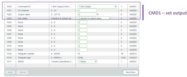
The most important is CMD 1, which is used to switch ON/OFF the output (0% => OFF; 100% => ON). The *Output value in percent* and *Dim value* is only applicable to devices with the dimming feature supported. The value 127% corresponds to 0x7F: Output value not valid / not applicable.
