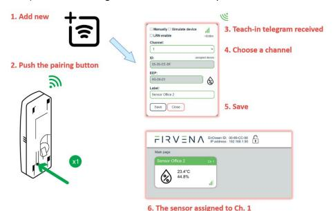
Optionally, the *Label* can be set for the device. The *Label* text is used in the *Channel labels* registers (see Ch. 8.2.5). If the *Label* field is left empty, the default text will be used.
