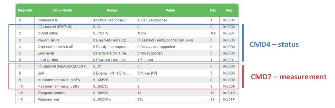
The most important is CMD4 -> Output value, which indicates the ON/OFF state of the actuator.
