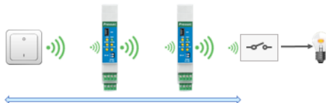
Fig. 2.9 Explanation of the Repeater enumeration
